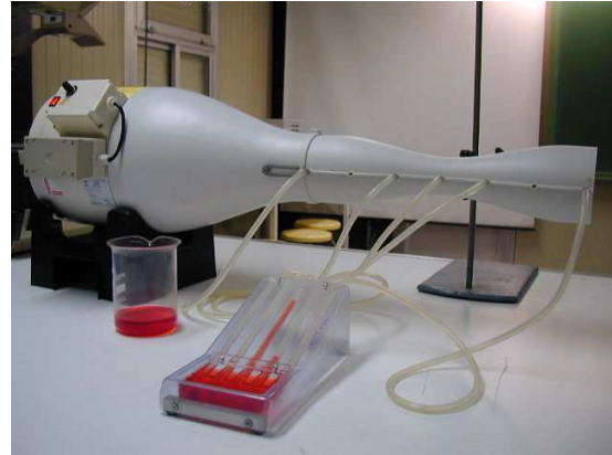
Figure 2: pictures of the container (left) and Venturi apparatus (right)
