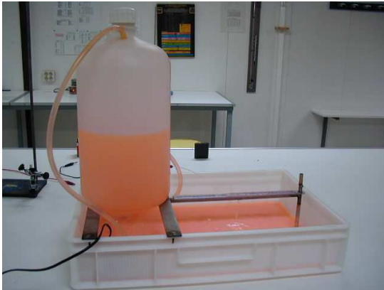
Figure 2: pictures of the container (left) and Venturi apparatus (right)
