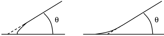
Fig. 5. Near the contact line, the LV surface deviates from the angle given by Young's equation ( \theta ) due to the finite range of the atomic interactions.
