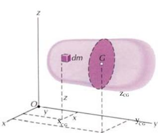
$$\vec{r}_{CG} = \frac{\int \vec{r} dm}{\int dm} \left\{ \begin{array}{l} x_{CG} = \frac{\int x dm}{\int dm} \\ y_{CG} = \frac{\int y dm}{\int dm} \\ z_{CG} = \frac{\int z dm}{\int dm} \end{array} \right.$$
