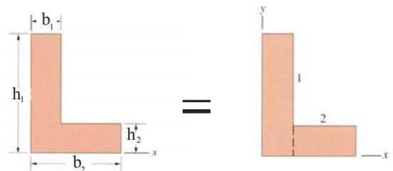
$$I_{e,x} = I_{e,x,1} + I_{e,x,2} = \frac{1}{3} b_1 h_1^3 + \frac{1}{3} (b_2 - b_1) h_2^3$$
